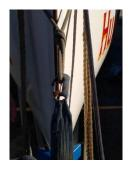
Put the rope tether through the fairleads on the bow of the Gig. Put the clip on the winch lead through the loop on the tether and use the winch to take up the slack on the tether. Use the ratchet stop on the winch to secure in position.
