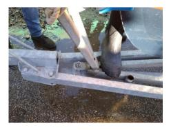
CAREFULLY slide the launch trolley and Gig along the road base until the slot on the launch trolley can be placed over the anchor post on the road base (you will have to lift the launch trolley again to do this.
